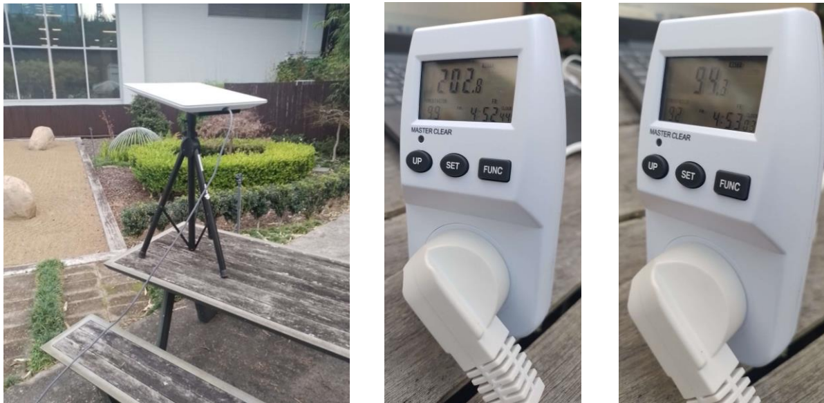
Figure 5: Set-up for the tests with the Starlink high performance unit, with power usage measurement (Test 5)
