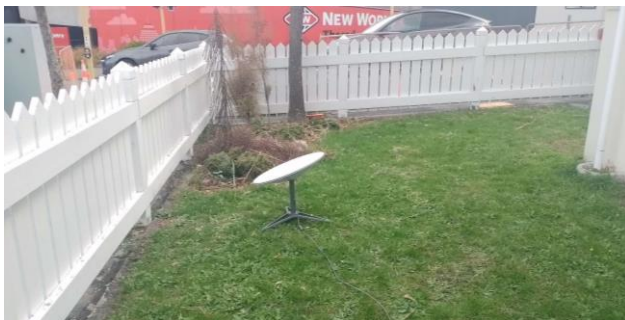
Figure 3: Set-up for the tests with the Starlink standard first generation unit (Test 3)
