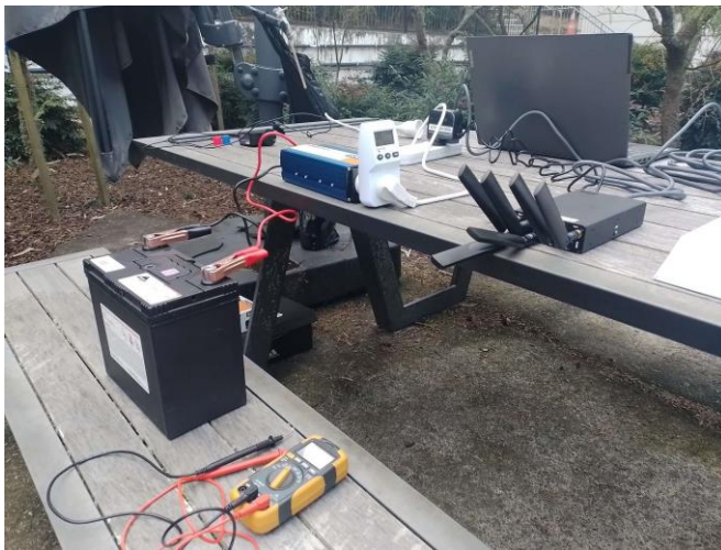
Figure 9: Set-up for Test 8, with battery/inverter as power supply
