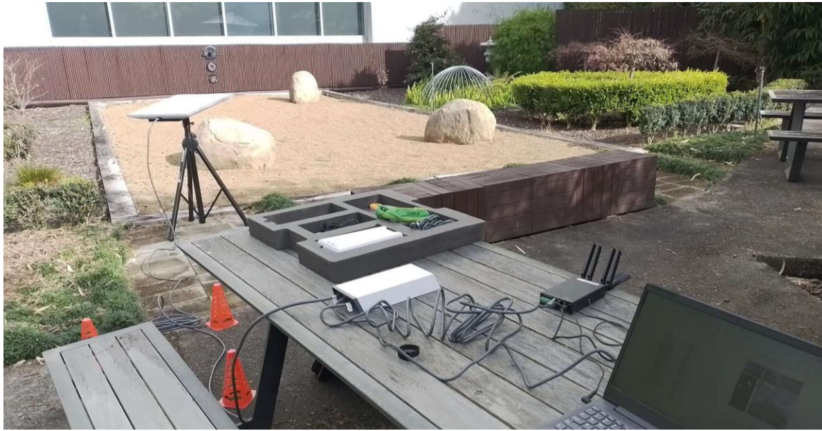
Figure 4: Set-up for the tests with Starlink high performance unit (Test 4)
