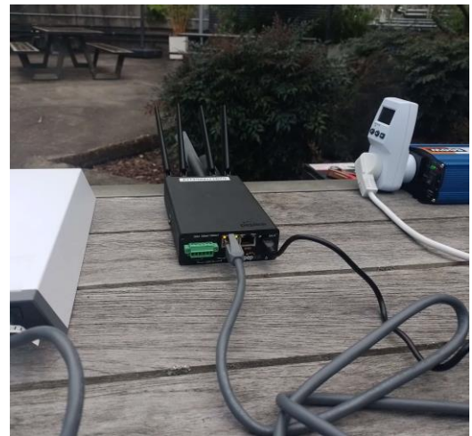
Figure 9: Set-up for Test 8, with battery/inverter as power supply
